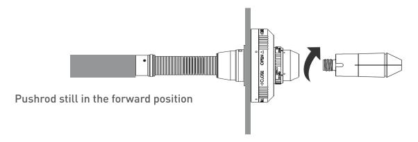
**NOTE**: Turning the blue sleeve from "Open" to "Close" moves a pin into one of the notches at the base of the collet, locking it in place. If you are unable to turn the blue sleeve fully to the "Close" position, you may have to turn the collet slightly. Conversely, if the blue sleeve is in the "Close" position but you are able to turn the collet, the pin is behind the collet and **you will damage it** when clamping your first tool blank.
