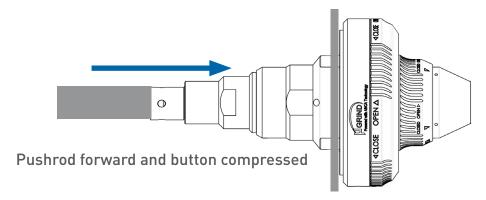
**Step 4**: Screw in the desired collet as shown in the video. Turn the collet clockwise until you feel resistance but do NOT tighten! Then turn the collet counterclockwise roughly 1/4 turn until the next slot aligns with the dimple on the chuck's nose. Turn the blue sleeve counterclockwise until the two "Close" indicators align with the dimples at the rear of the chuck's nosecone. Check that you are now **unable** to turn the collet more than a tiny bit in either direction.
