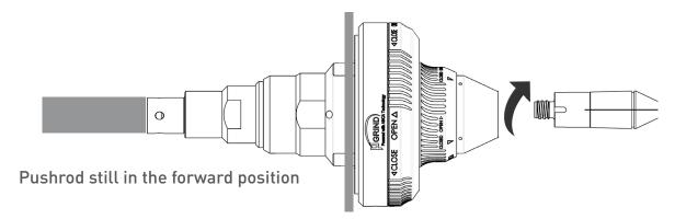
NOTE: Turning the red sleeve from "Open" to "Close" moves a pin into one of the notches at the base of the collet, locking it in place. If you are unable to turn the red sleeve fully to the "Close" position, you may have to turn the collet slightly. Conversely, if the red sleeve is in the "Close" position but you are able to turn the collet, the pin is behind the collet and you will damage it when clamping your first tool blank.
