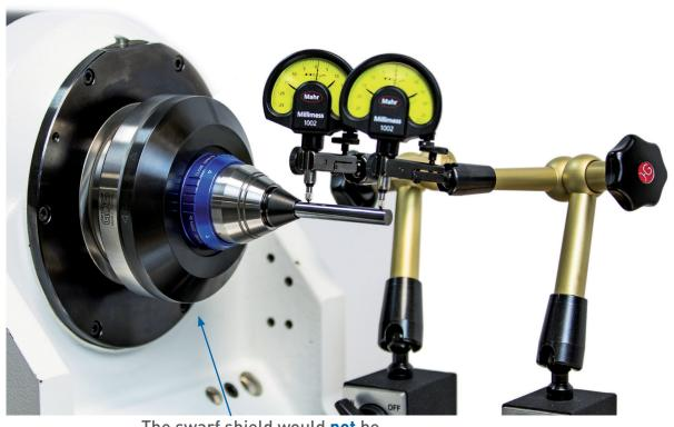
The swarf shield would **not** be on while adjusting the chuck
