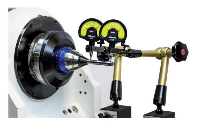
**Step 7**: As shown in the video, use the plastic tipped mallet supplied with the chuck to "tap down" the runout. Rotate the A-axis periodically to ensure that you have achieved the desired precision. Tighten the face bolts when satisfied.
