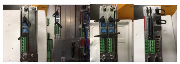
You need to check and set the SERCOS interface (fibre optic) transmission speed and capacity. The three drives pictured on the left all have the same SERCOS card. All these cards are identical except the axis address (little blue turn switches). They also have 3 DIP switches inside that must to be set correctly.
