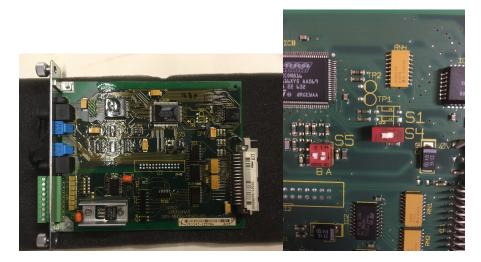
On double drives with a glass scale interface the SERCOS card is built in and the DIP switches are in the drive. See the picture below with location and settings.
