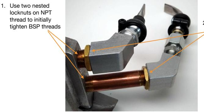
Then use locknuts to lock position of the NPT thread as shown. Use Teflon tape to seal the threads
