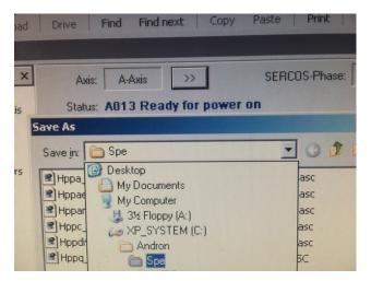
9. Give the file a clear name. For example #axis# - #machine number# - optional #date# (In our example it's the A axis of machine 65000)
