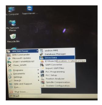
5. The drive data software gives you access to every single drive and the parameter set. The default page is always the lowest address – "axis A" (If you need a different one select it with "F9 – axis")
