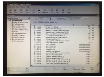
6. To save the drive data, use the pull down menu, which you open with "Alt" and than "File – Save As..."
