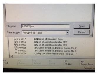
10. Select "Save" and start with the Enter command. A window pops up in which a bar runs from left to right while the parameters are being saved.
